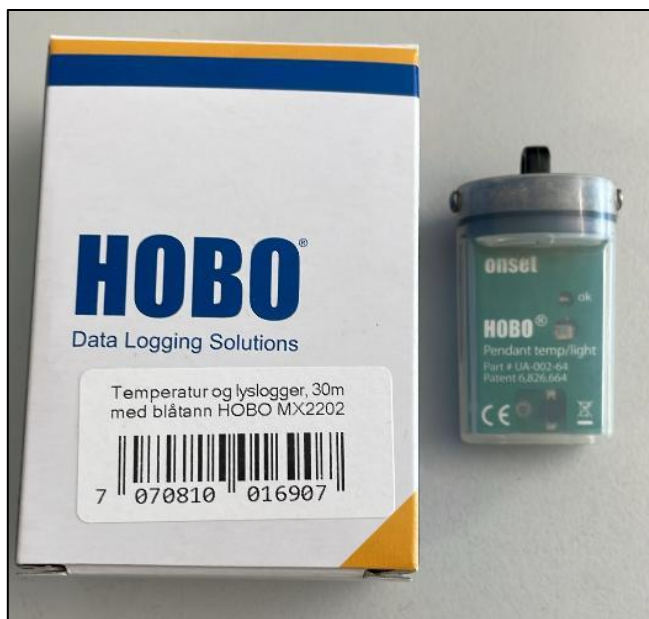
Figure 6. The temperature and light logger that was used in the study. During the study there were two HOBO loggers, one at 1 meter, and a second at 2 meters. This was to ensure a more robust data collection.
