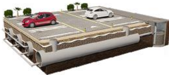
Figure 6. Typical solution with pre filtration to remove organics and a final filter with Filtralite® HMR.
