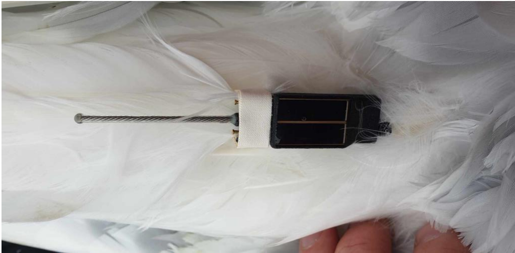
Figure C1: PathTrack nanoFix®GEO + RF tag. Secured with cable tie at the base of the four middle tail feathers and tesa tape at the end. Photo: Author.
