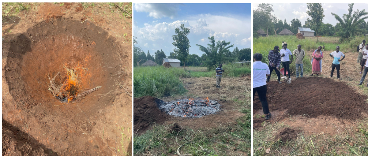
Figure 1. Open flame Kon Tiki method of biochar pyrolysis in Gulu, Uganda. Photos: Mathilde Brunvoll
