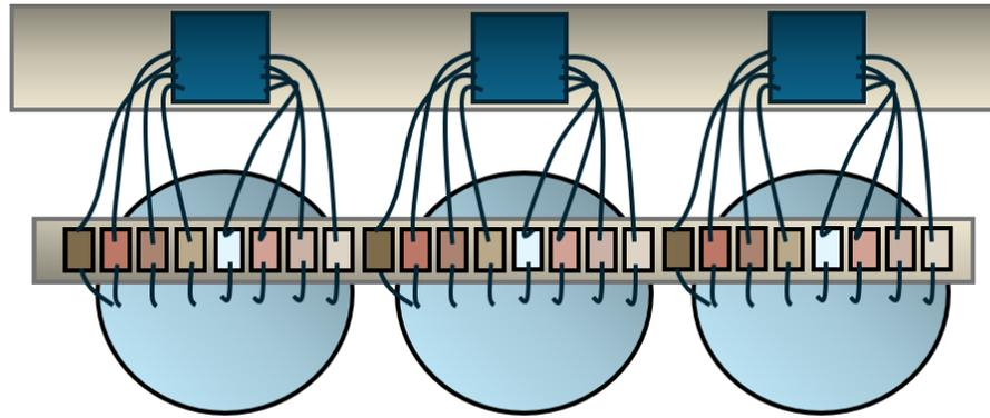
*Figure 1 Illustration of the recirculating system. The system consists of a series of reservoirs linked to a central header box, which distributes water uniformly across eight containment units. This design simulates a riverine ecosystem with a continuous flow of water, ensuring consistent environmental conditions.*
