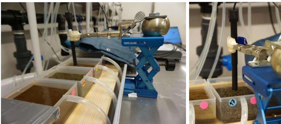
Figure 6 Illustrates the setup featured an O<sub>2</sub> microsensor (Unisense A/S) with reinforced steel needle (3-5  $\mu\text{m}$ ). It incorporated a specialized adjustable lift table with a grab mechanism, allowing for precise positioning and stability.
