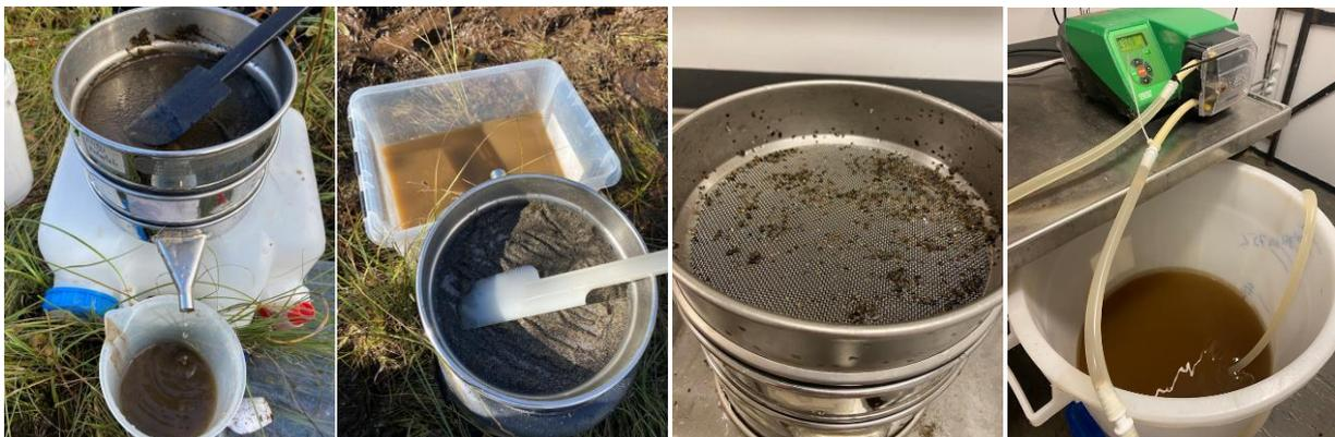
*Figure 4 Images of sediment treatment procedures and sieving analysis. The two pictures on the left display the sediment treatment process during sample collection in the rivers and the sieving analysis. The two pictures on the right show the sieving analysis, featuring both the sieve and the pumping mechanism used to differentiate between clay and silt.*
