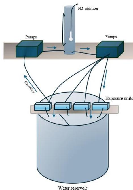
*Figure 5 Illustrating the setup features a 100 L reservoir supporting four experimental boxes. A 65 x 12 cm cylinder with a nitrogen pump maintained low oxygen levels. Two peristaltic pumps coordinated water flow: one directed water to the cylinder, and the other regulated flow to the experimental boxes. A silicon tube outside the cylinder displayed the water level, ensuring accurate monitoring.*
