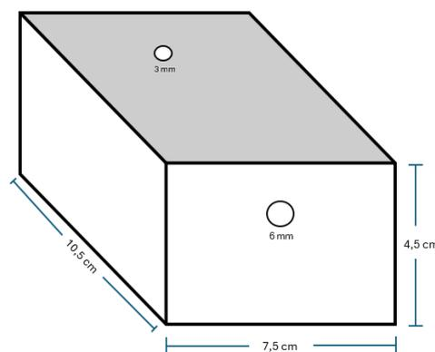
*Figure 2 Illustration of the experimental boxes. Each box with standard dimensions, and two drilled holes.*
