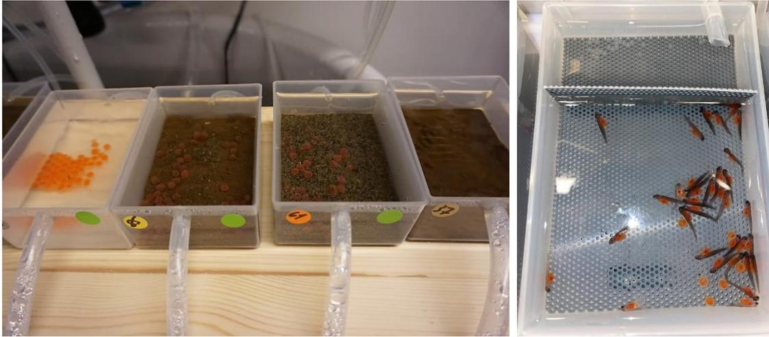
*Figure 3 Shows photos of sediment exposure boxes with control unit (left) and sediment units (centre), alongside the oxygen exposure unit (right). This setup illustrates part of the experiment arrangement used to study sediment and oxygen effect.*
