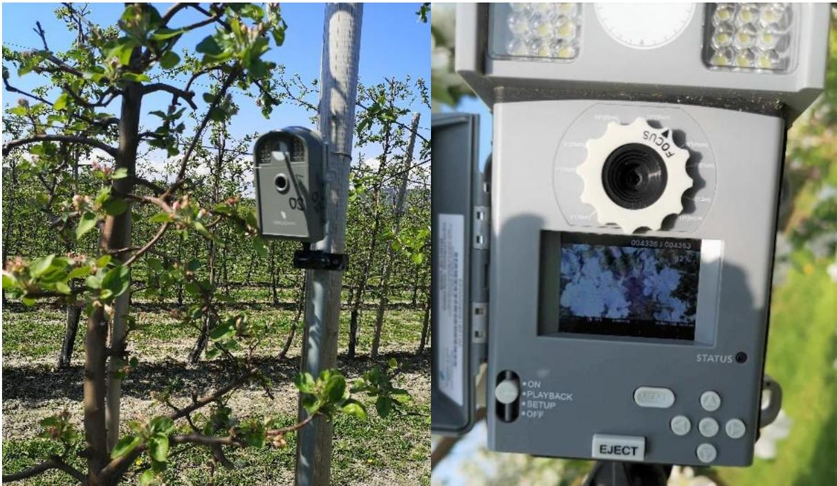
**Figure 5.** Left: field-camera mounted on a wood-post in the orchard. Right: field-camera focused on apple flowers.
