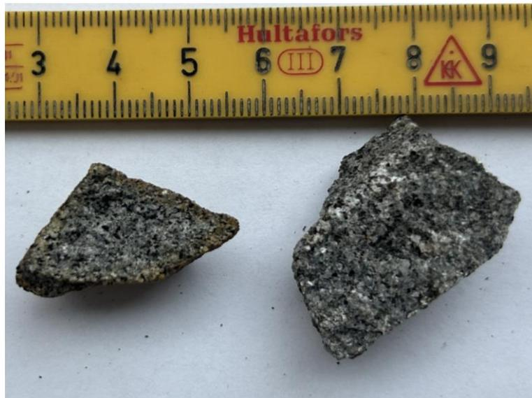
Figure 13: Tingsaker skole #2, to the left the stone piece might be weathered as there is an orange colour in the outer corners.
