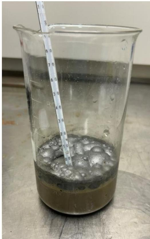
*Figure 10: Setup for the Agder method. The sample reacted visibly as exemplified by the formation of bubbles (steel grey colour) and generation of heat.*
