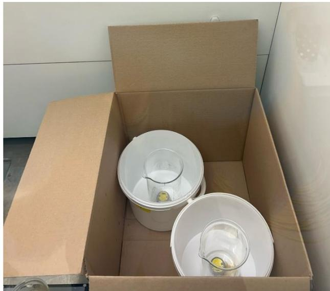
*Figure 9: Experimental design for single NAG test. The white buckets with beakers and temperature loggers are placed in a cardboard box. The cardboard box is closed during the experiment.*
