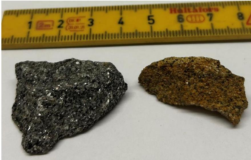
Figure 15: Sample Tingsaker skole #3. The piece to the left is fresh surface and has no sign of weathered surface. The piece to the right is rusty in the colour, and crumbles when touched.
