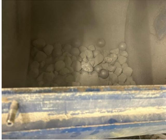
*Figure 7: Inside of the Los Angeles crusher. Steel balls that are rolled together with the gneiss sample.*
