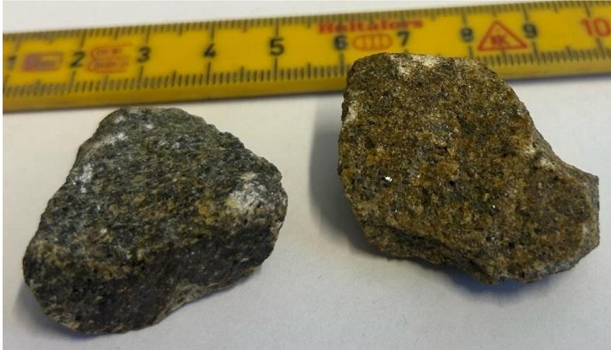
*Figure 22: Rock sample Arendal legevakt 2. The piece to the left is less weathered and has the freshest surface that is grey. To the right is more weathered and are more rusty orange coloured.*
