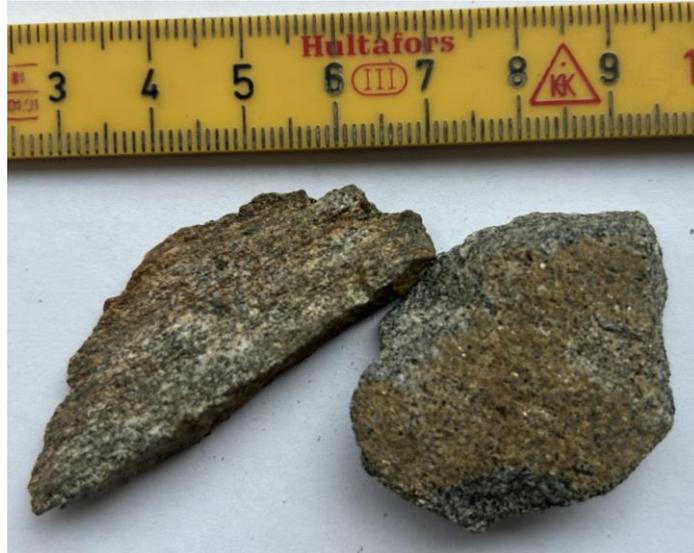
Figure 20: Nordbø 1 has more weathered surface, but there are some spots inside the gneiss that is weathered.
