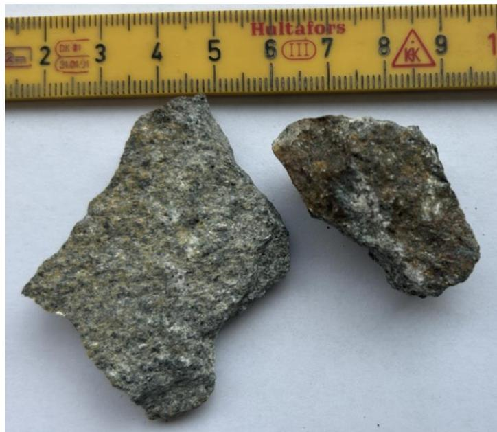
Figure 21: Groos 1, the piece to the left shows the grey fresh surface colour and the orange weathered colour. The piece to the right shows piece with reddish colour.
