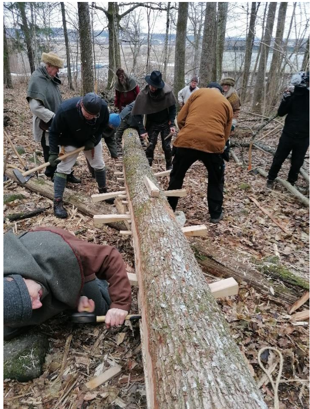
Figure 18, The spanning fibres are cut in the open portion of the split-crack. Here the practiced hand of Jan Vogt Knutsen works swiftly and helps tension be further focused on the remainder of the connective fibres, While Tore Forsberg, facing away, being filmed, deftly and rhythmically drive wedges together with the volunteer workers. Photo by Author.
