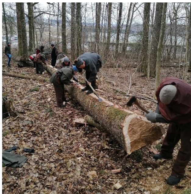
Figure 14, A strip of bark is being removed, to enable the marking of the splitting line along its length. At the same time the cut-face at the root-end is cleaned up. A choir of scraping and small knocks is heard when the work is ongoing. Photo by Author.
