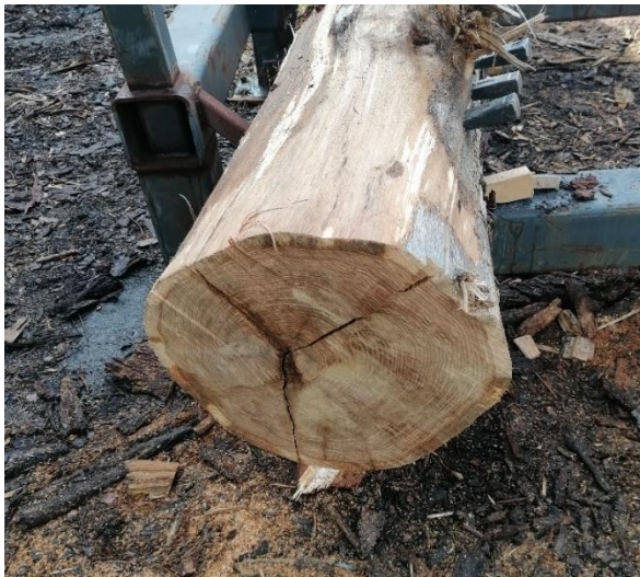
Figure 9, Log nr 4 of subset 2. A split-crack gone past the pith into an already extant crack that was presumably created from the handling of the log.
