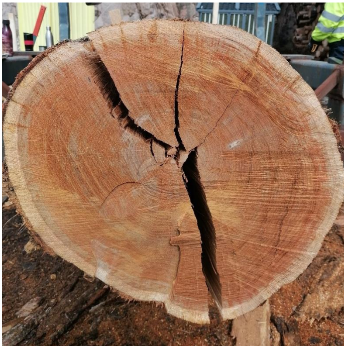
Figure 11 Log nr 4 of subset 2, The split-crack is extending as far as it is able, Without a group of wedges on the other side to act as a guide, the split-crack opens ‘willy nilly’, even forking and “shattering” the cross-section. A palpable dissatisfaction is voiced by the team of amateur cleavers, me included, at this result.
