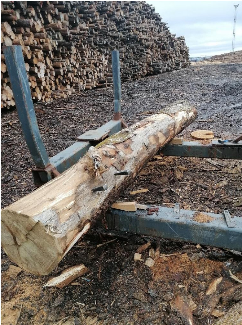
Figure 8 Log nr 4 of Subset 2. Laying initiated and ready for cleaving, metal wedges have already been struck into the points along the initiated line from which the cleave will proceed. Namely at the most critical points from which failure or success is achieved. Note the clear proximity to the broken branch. Picture taken by Author.
