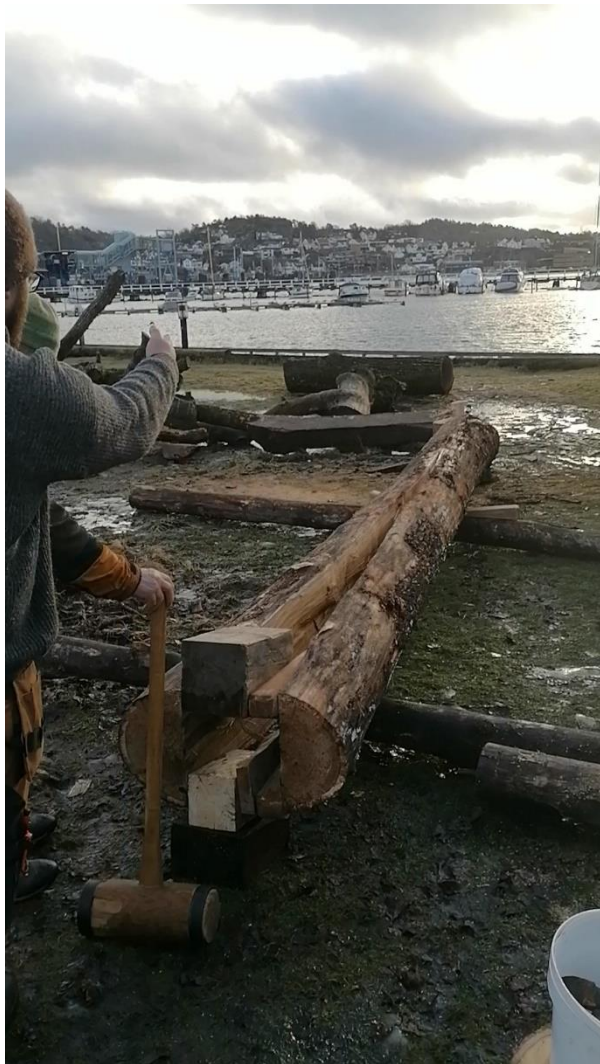
Figure 7, Log nr 1 of subset 1 is allowed to rest after being pressured, the sound of crackling tension being released is continual as it nears the completed split by itself. No further strikes are necessary before this log splits open on its own. Picture taken by Author.
