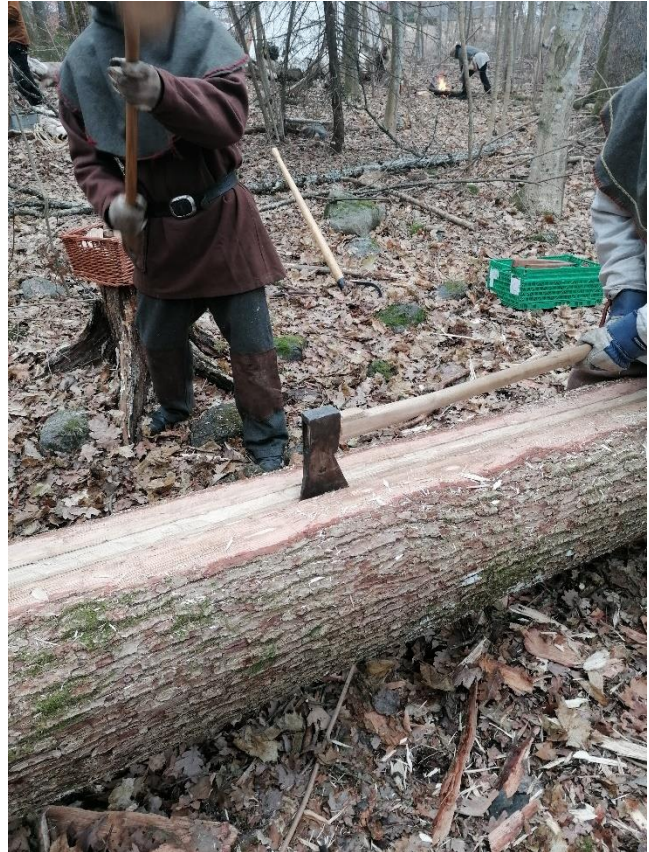
Figure 15, The log is initiated along the bottom of the first v-groove. The early birds do the work, as the rest of the work-team prepare their tools and start fires for the day. Photo by Author.
