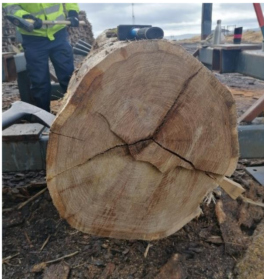
Figure 10, Log nr 4 of subset 2 Wedges are starting to be driven from the other side to prevent this development from spreading further down the length of the log. A handaxe at the end of the initiation process is seen having produced the pre-cursor to the wanted
