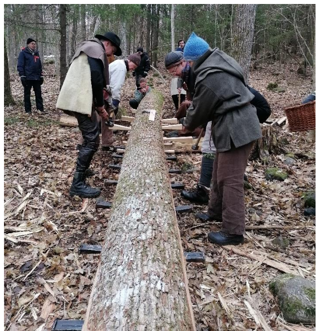
Figure 17, Cleaving has begun in earnest, workers stepwise introduce larger wedges, before they're brought further and further forwards, notice the root-end of the log has no wedges, as they have all been moved. Photo by Author.
