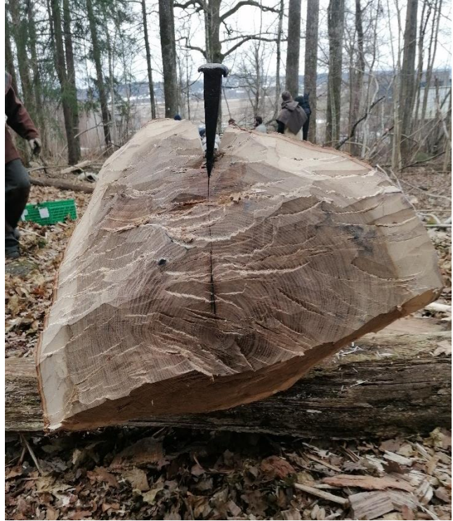
Figure 16, The first strike on the first wedge produces a straight split-crack to the pith. The log is turned and initiated from the other side, before any more are driven. Photo by Author.
