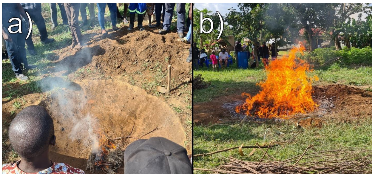
Image 1: a) Start of pyrolysis process in a Kon-Tiki flame curtain kiln in Uganda. b) Flames in the pit consume most oxygen before it reaches a lower level of the kiln. Photos by Adrian Røed Østby.
