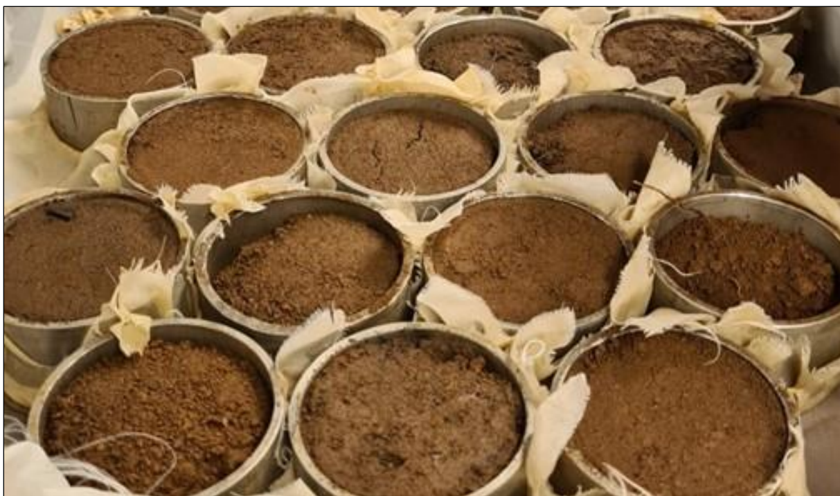
Image 4: Example of core rings with varying levels of missing soil. Photo by Adrian Røed Østby
