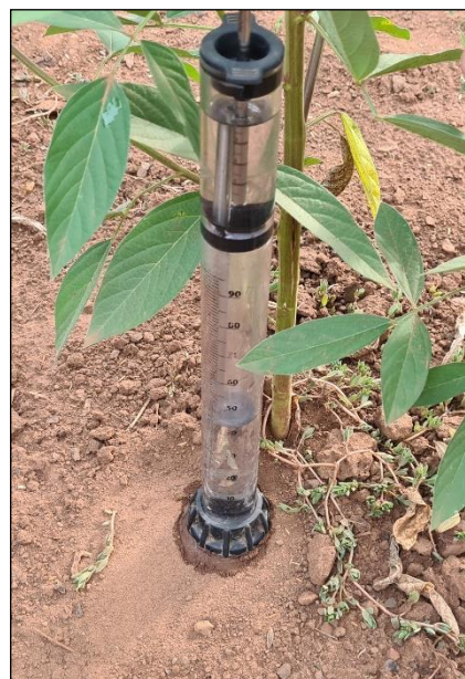
Image 2: Mini Disk Infiltrometer in use at - 4 cm pressure. Photo by Adrian Røed Østby.
