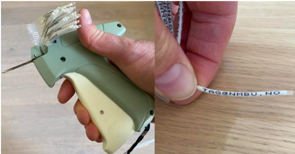
Figure 6. Photograph of the tagging equipment used. Mark III regular tagging pistol with a heavy-duty needle (left) and external Floy tags with a university email address on (right). Photos: Jonathan Colman.
