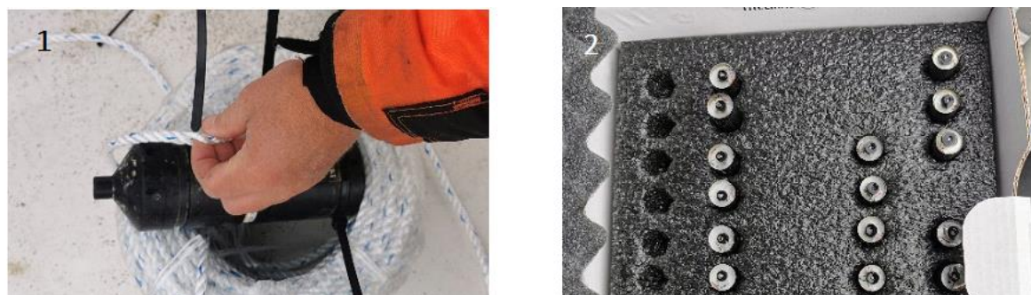
Figure 3. The method of acoustic telemetry requires a transmitter to send sonic pulses and a receiver to receive and store the detection. 1: A receiver being attached to a rope. 2: Multiple transmitters. Both the receiver and transmitter are produced by Thelma Biotel AS, Norway.
