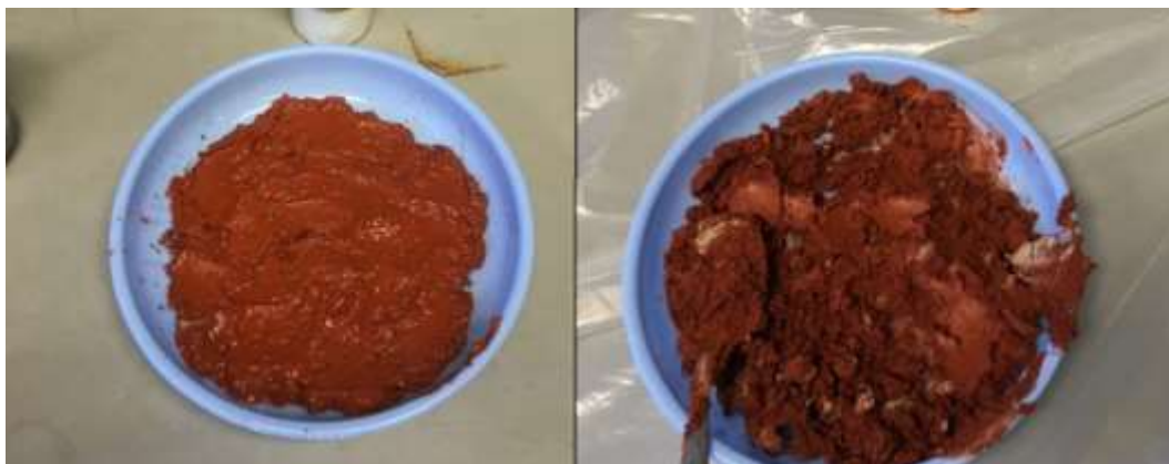
Figure 4. 10 Photographs taken of BR (left) and BR+10% gypsum (right) immediately after taking down the columns, three days after the last water addition.
