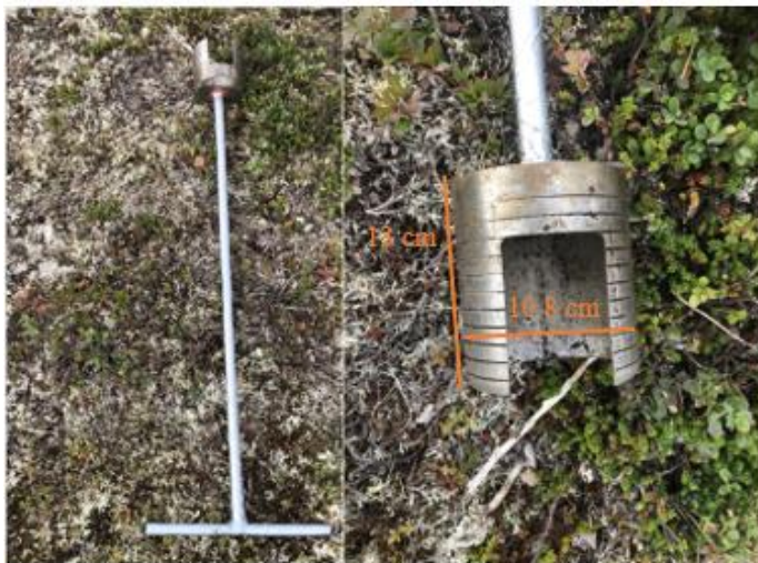
Figure 3.6: The soil sampler corer. The diameter and depth of the corer are shown.
