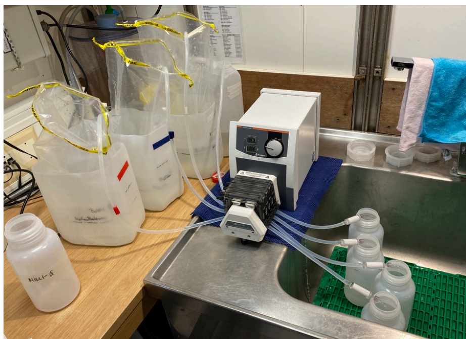
Figure 2 Picture for demonstrating the sampling procedure. Filtering of water samples from cruise onboard Kristine Bonnevie March 2022. Here special plastic bags were used instead of using water canisters to collect water from the CTD.
