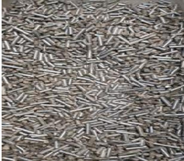
Fig 2. Pellets of digested sludge
