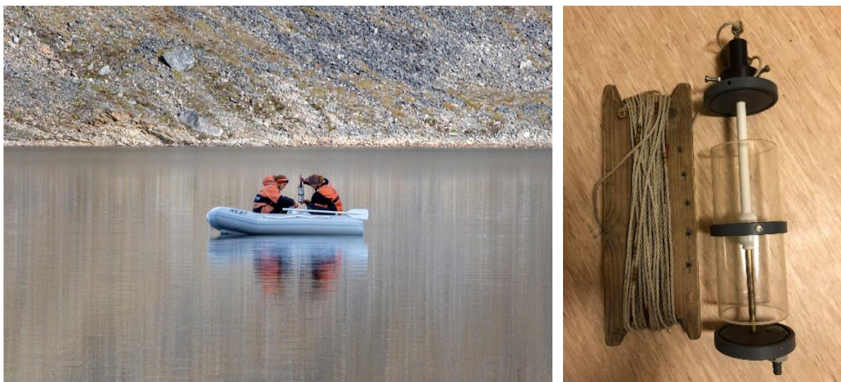
Figure 6: Left: Water sampling from various depths in Lake Sarsvatnet. Photo: Sunniva Kvamme. Right: Water collector used to obtain water samples in the lake. Photo: Lill Katrin Gorseth
