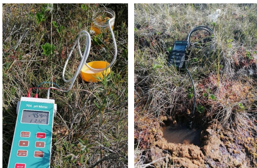
Figure 4. Left: pH was measured by first collecting water in a container, and then submersing the measuring cell of a pH meter into the container. Right: Electrical conductivity (EC) was measured by submersing the measuring cell of conductivity meter directly in the bog water.
