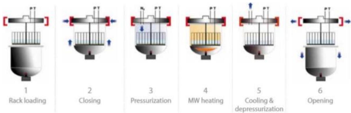
Figure 6: The automated steps of the UltraClave process. Source: (Automated, n.d.)
