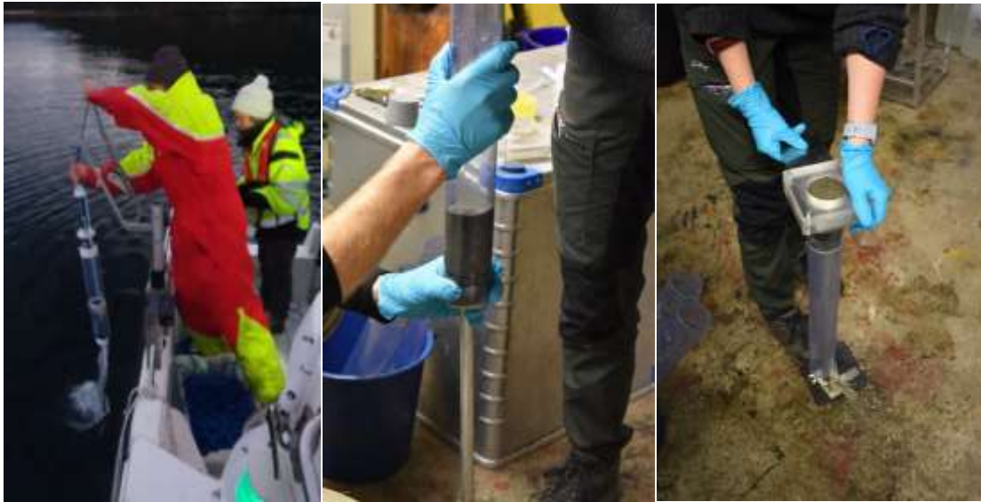
Figure 3.5: Sampling and slicing of sediment core.
