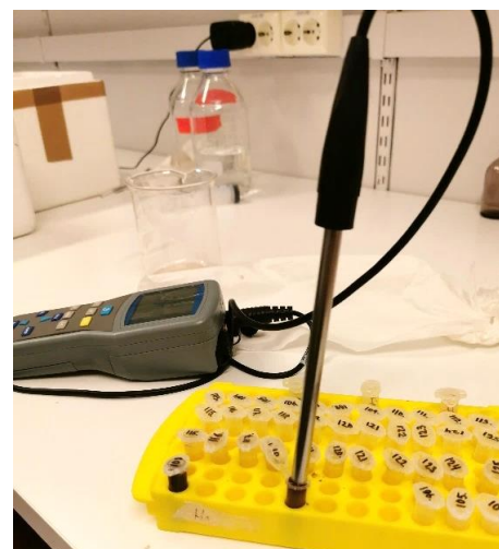
Figure 14: Photograph of how pH was measured in 0.5 ml slurry
