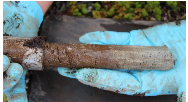
Figure 9: Photograph of the bottom of the PF core sampled at Lakselv, showing the transition of organic to mineral soil
