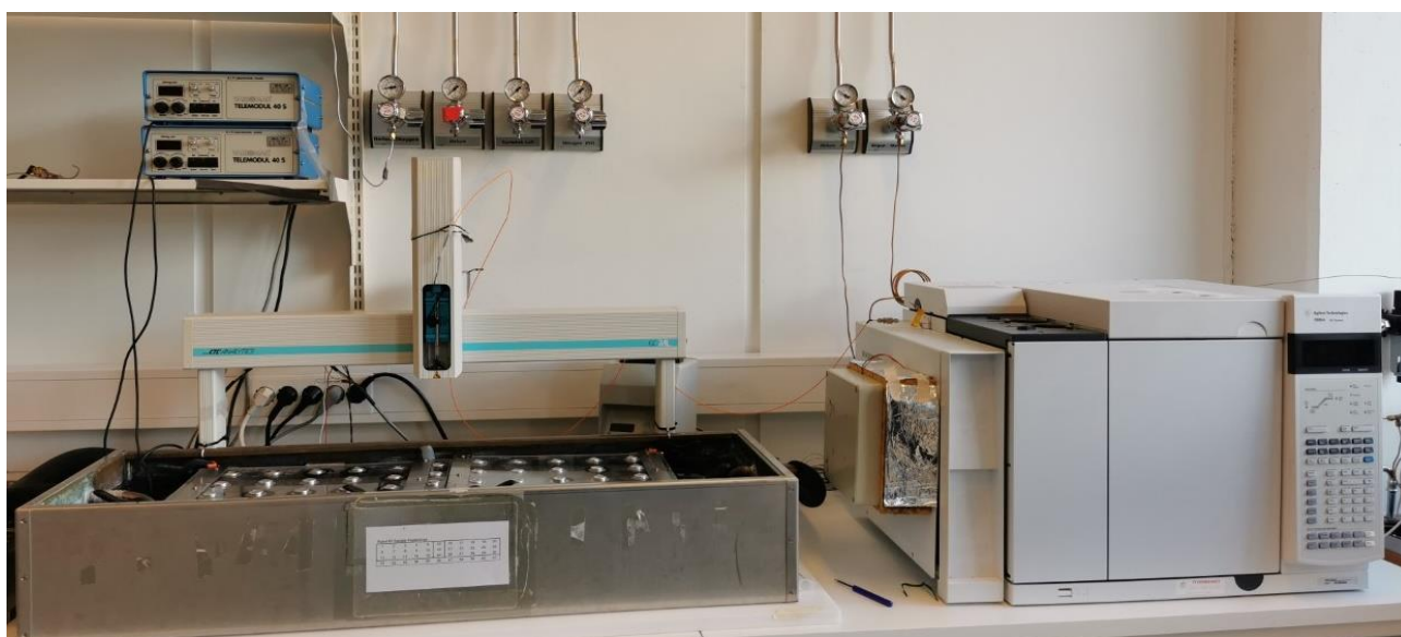
Figure 12: Photograph of the automated incubator used in the study; The unit consists of a temperature-controlled water bath with submersible stirring boards, a freely programmable autosampler periodically piercing the septum bottles with a hypodermic needle and a peristaltic pump transferring ~1ml headspace to a multi-channel gas chromatograph with loop injection
