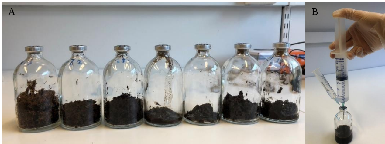
Figure 13: Photographs of loose and slurry treatments. A: A depth profile from Işkoras in serum bottles. From left to right: AL1, AL2, AL3, TZ, PF1, PF2, and PF3. B: Creating the slurry by adding ultra-distilled water through the septum with a syringe, while releasing overpressure through a syringe without plunger but filled with water to prevent air from entering the bottle
