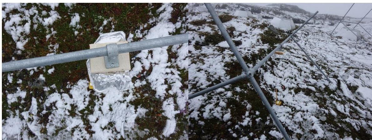
Figure 2: The cameras were mounted to a wooden plate and protected by an improvised housing of aluminum foil. The cameras were then mounted to a horizontal bar between a double A-frame. Five of these were placed at each site.
