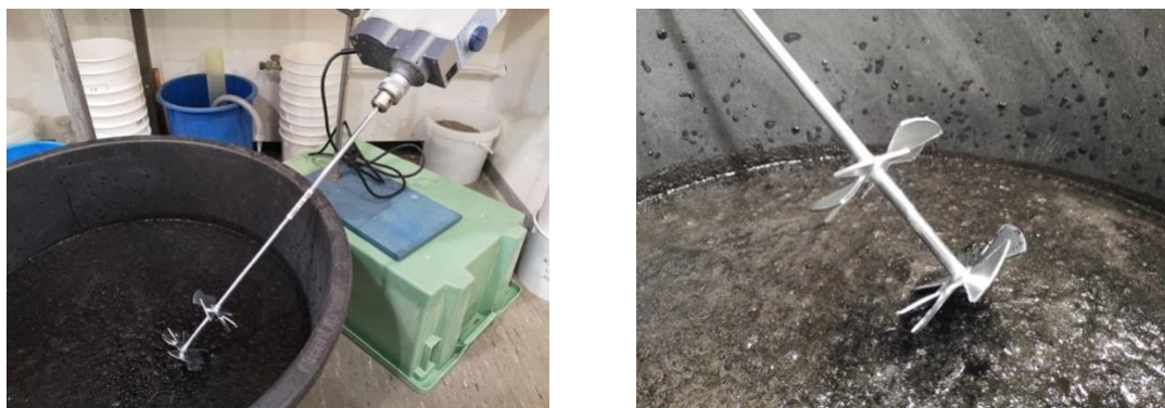
Figure 3.3. Mixing equipment used for the washing and enriching of biochar
