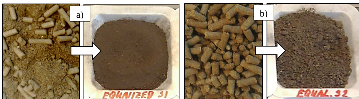
Figure B.5 Source material for TS and VS measurements: a) Lindum/Vesar WS; b) Ullensaker WS
