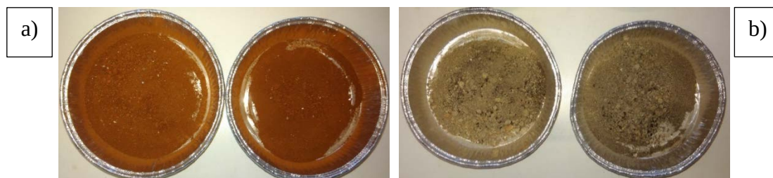
Figure 5.1 – Source material after ignition: a) Lindum/Vesar WS; b) Ullensaker WS
