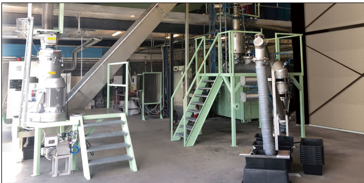
Figure 4.2 – Microwave-Assisted Pyrolysis system (MAP) (Scanship AS, 2019)
