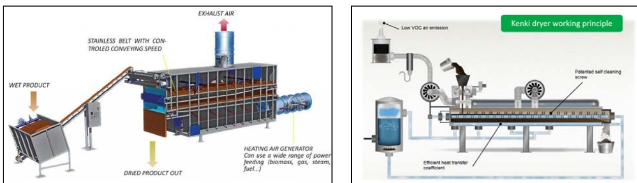
Figure 4.1 – Equipment for biomass drying: a) continuous belt dryer; b) KENKI dryer (Biogreen®, 2021a, 2021b)
