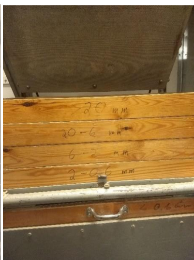
Figure 2.9 – Motorized sieve. Photo: Thomas J. Brown (2021).
