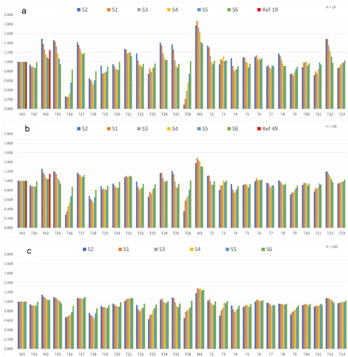
Figure 17 Normalized wind speed for all turbine positions in cases S2-S6. Displayed here for heights 19 (a), 49 (b) & 100m (c) above the terrain
