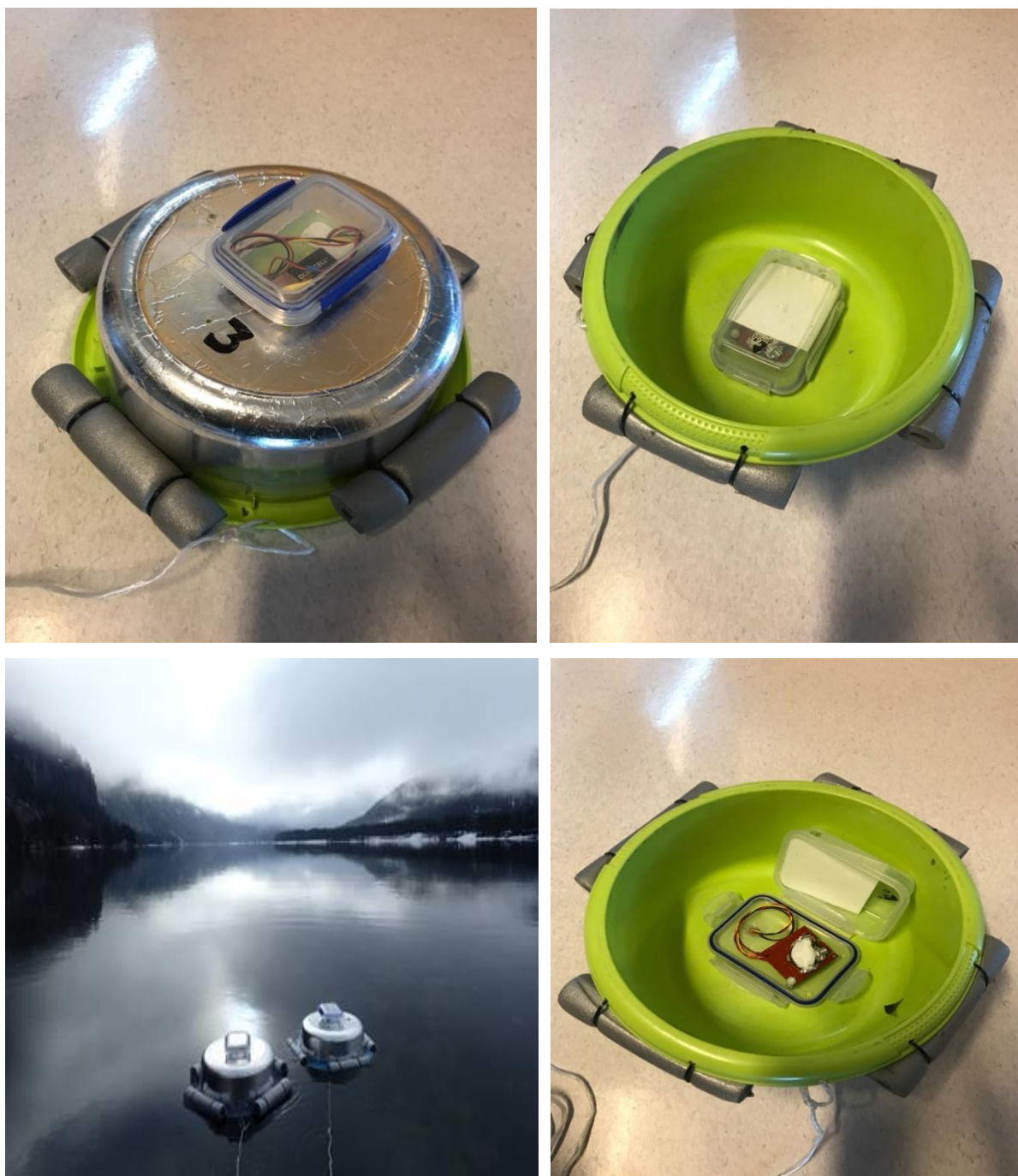
Figure 2. Pictures of the floating chambers with Infrared Gas Analyser (IRGA) with CO 2 logging abilities. Used to measure CO 2 emissions.
