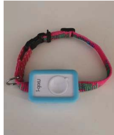
Figure 2: i-gotU GT-120 attached to a simple cat collar
