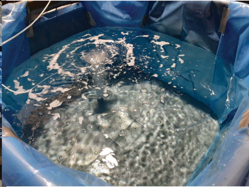
Figure 3.2 Tank lined with plastic wrapping with aeration stone. Photo: Emil Jarosz.
