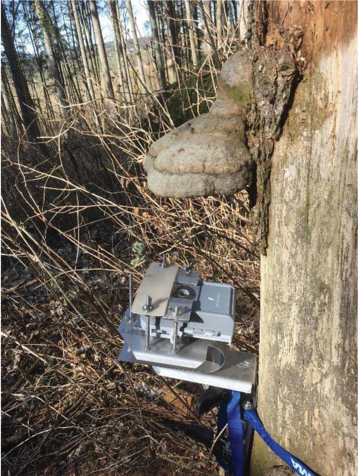
Figure 2.2. The camera setup used in this project. A time-lapse camera is mounted to a spruce trunk at an angle, taking a picture of the sporulating surface every ten minutes. The photo was taken at a test site that was not in the final project. Photo: Tone Birkemoe
