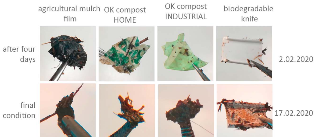
Figure A6: Visual examination of the 1.5L incubation at 55°C. None of the biodegradable plastics have started fragmenting or degrading in the period of 20 days.
