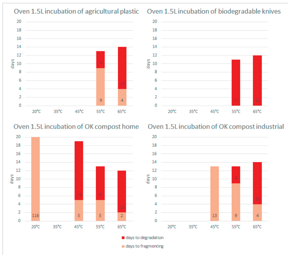
Figure A8: Days to fragmentation and degradation of biodegradable plastics in an oven at indicated temperatures and sorted by temperature. Zeros refer to the process not being observed rather than missing data. The numbers in each category indicate the number of days that passed until it reached the next state. For example, agricultural plastic at 55°C began to fragment after 9 days and has shown first signs of degradation 4 days later. Note that room temperature is on a different scale than other temperatures.
