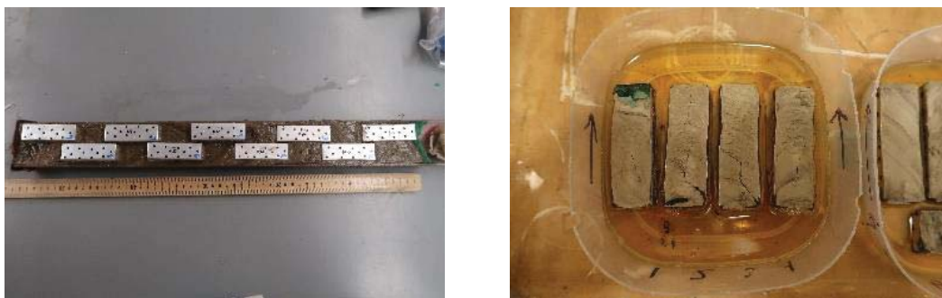
Figure 4.2: Left: the boats are pressed down into the sediment along with the core in an alternating left-right pattern with 1-2 cm overlap. Right: Epoxy-resin was poured carefully in the corner of the plastic box and did not cover the subsamples.
