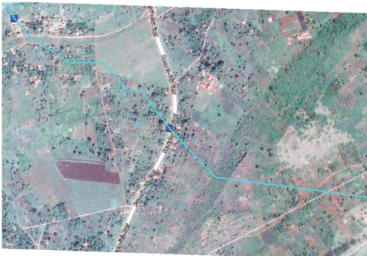
Figure 21: Map of groundwater flow path into the well of Nyenga foundation (blue square in left upper corner). The flow path goes through the well of the chairman (blue square in the middle). The chairman well is at split 50 ca.1200m in Figure 22. The flow path is manually drawn and may be different out from geological conditions.
