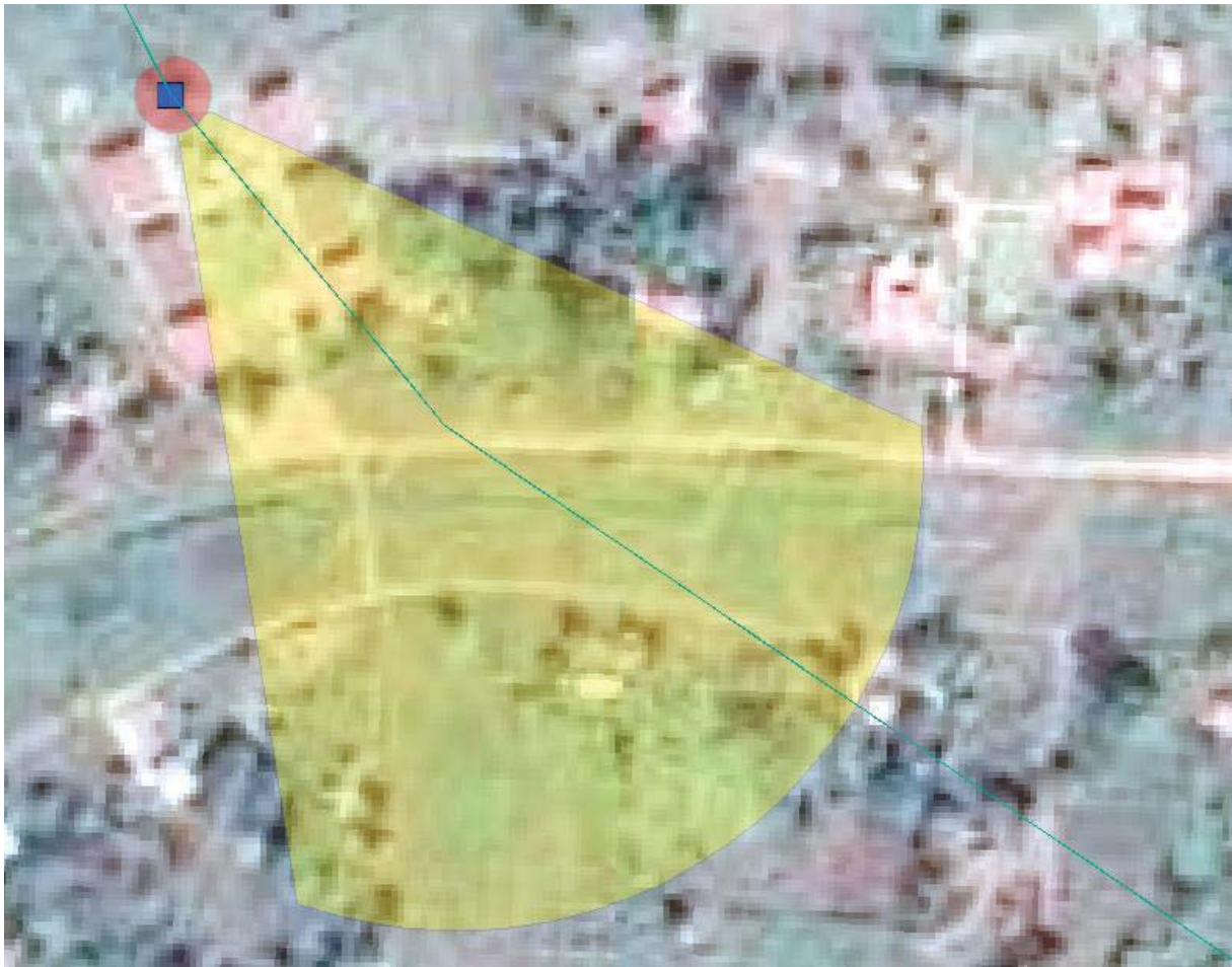
Figure 24: Risk map. Nyenga foundation well is placed at blue square while blue line is flow path from Figure 21. The red area shows the area regarded as high contaminant risk (10m). The yellow area shows a theoretical area of contamination out from the uncertainty of T and S (208m). The risk area is a subjective area out from the topographic characteristics in the area and may be larger due to geological features.
