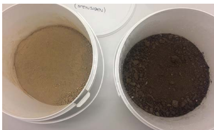
Figure 12. Soil samples after homogenization and sieving (16 mm). Left: The shooting range soil. Right: The urban soil.
