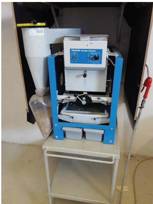
Bilde 17 viser Pfeiffer Sample Cleaner rensemaskin for kornprøver.
