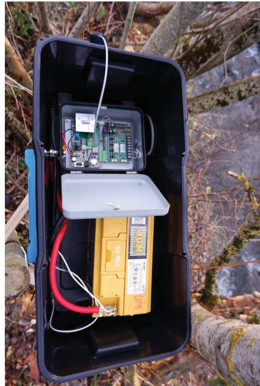
Figure 5: The container with reader box and battery.
