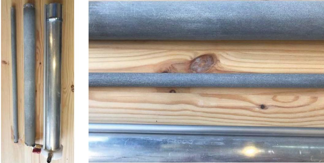
Figure 39. Appearance of electrodes after all the tests
