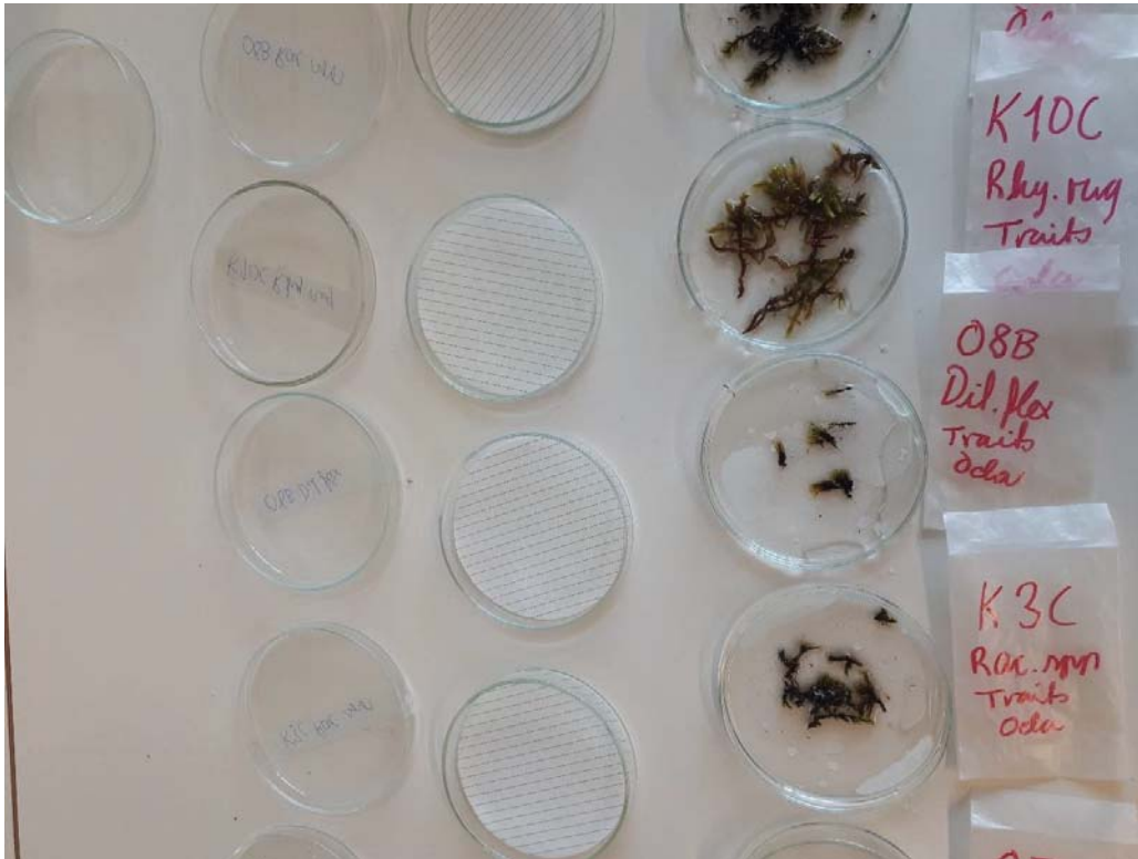
Figure 5: In the process of measuring water holding capacity (WHC). Sampled shoots in the process of soaking before 24h incubation and weighing.
