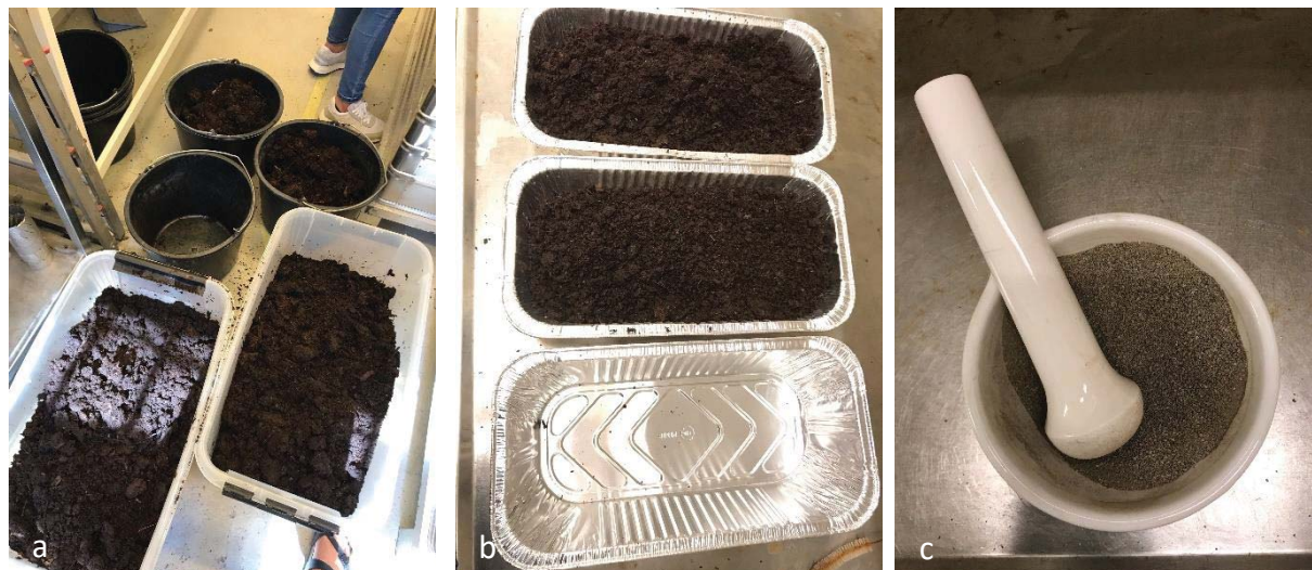
Figure 6a-c): Soil sample preparation, a) initial homogenisation of total soil sample, b) homogenisation of soil subsample, and c) crushing of soil sample.
