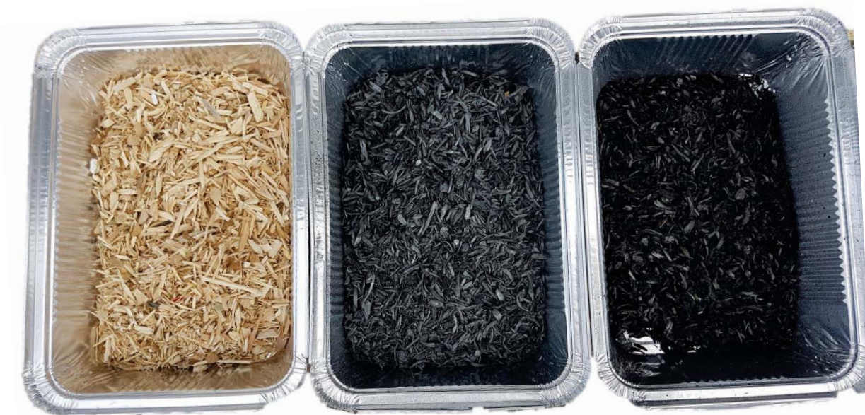
Figure 7: Three stages of biochar production; shredded waste timber (biomass feedstock), biochar, and activated biochar (from left to right).
