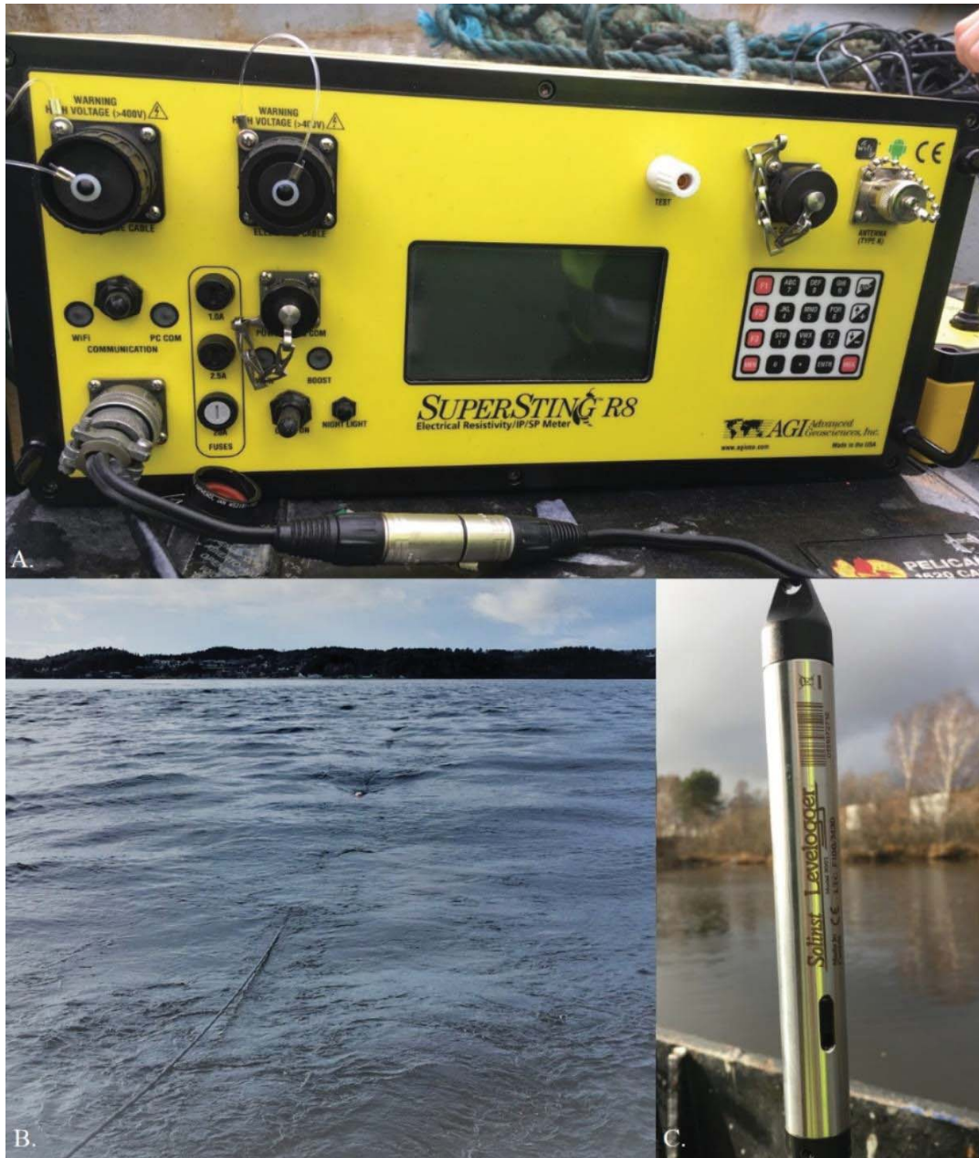
Figure 10: Show some equipment from the fieldwork. AGI SuperSting R8 (in picture A), the cable with electrodes towed behind the boat (B) and Solinst Levellogger (C).
