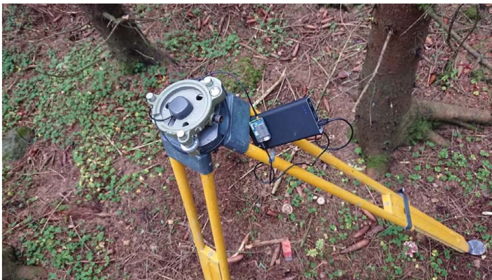
Figure 7: Setup for GNSS data collection, Emlid Reach
