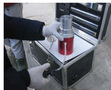
Figure 59: Pumping water sample through a 45µm filter paper
