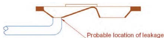
Figure 169: Connection between urine-diverting pan and urine pipe which is prone to leaking (WaterAid, 2011)
