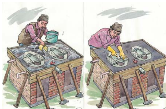
Figure 155: Cleaning of a UDDT (ENPHO, n.d.-a)
