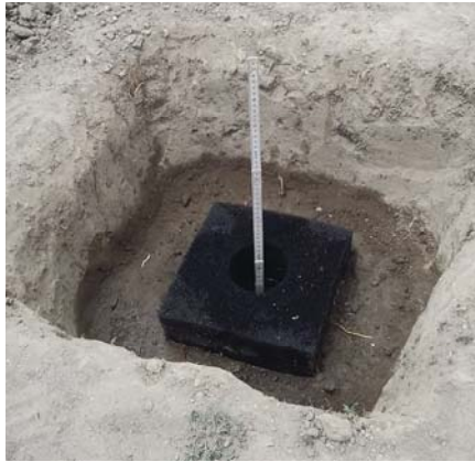
Figure 54: Running infiltration test at site 1
