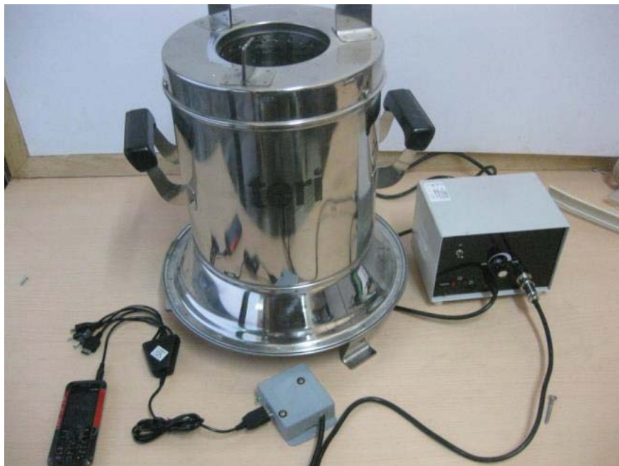
Figure 4.6: Stainless steel forced draft cook stove developed by TERI (TERI, 2016)
