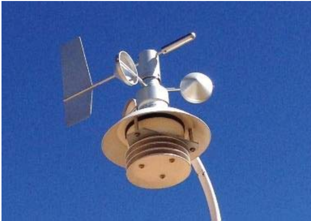
Figure 3-3: The MetOne weather station. Photo: Mari Øgaard, with permission
