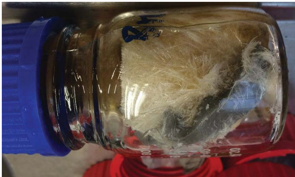
Figure 21: Crystallization of \text{H}_2\text{O}_2 solution at -20\text{ }^\circ\text{C} when left in freezer for longer than 45 min
