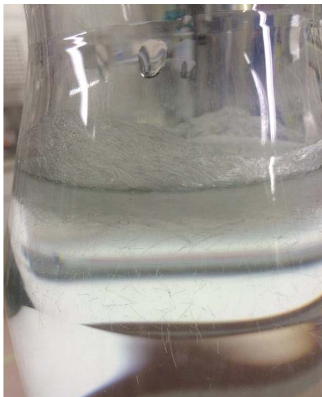
Figure 26: (Left) PE fibers stuck to the Bauta glass column wall at the constriction when introduced in the sediment chamber. (Right) Distribution of PE fibers in the solution column.
