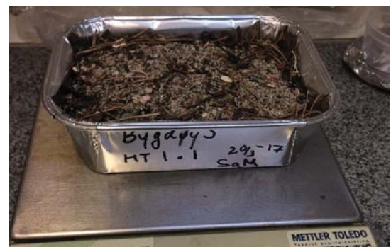
Figure 12: Sample distributed in pre-weighed aluminum trays and weighed before oven-drying at 60 °C, 24h
