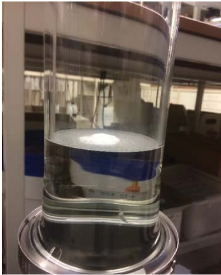
Figure 25: (Left) Introduction of PE powder in the separation chamber. \text{CaCl}_2 solution is filled from the bottom.
