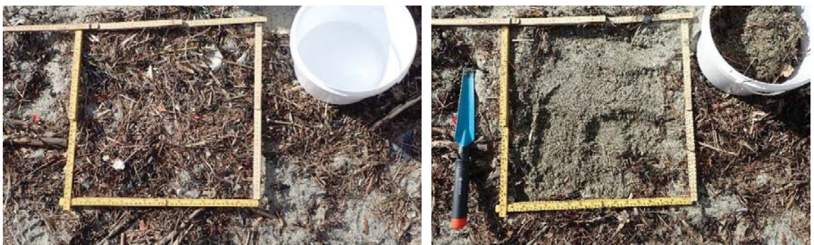
Figure 8: (Left) Demarcating 40 \times 40 \text{ cm}^2 on the HWM before sample collection
