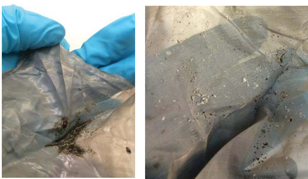
Figure 34: Before (left) and after (right) chemical digestion of sediment sample F1 on steel mesh (45 \mu m)
