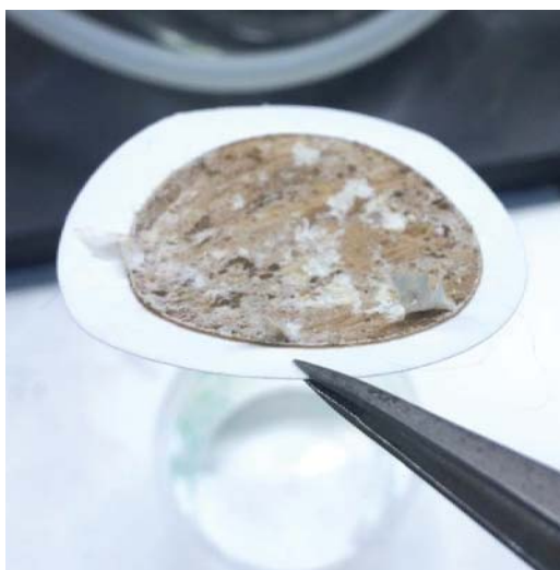
Figure 29: Precipitate of \text{ZnCl}_2 : \text{CaCl}_2 on GF/C glass fiber filter paper during method optimization.
