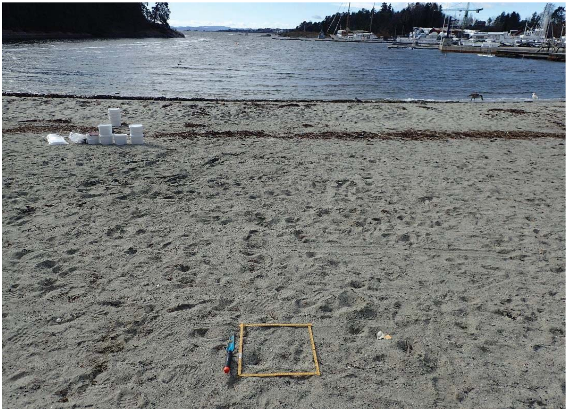
Figure 7: Sampling site in Bygdøy sjøbad. A wooden ruler is placed marking an area of 40 \times 40 \text{ cm}^2 on one of the sampling points on HWM+6m. Further towards the sea, the HWM can be distinguished by the presence of debris accumulated. The HWM-6m, nearest to the sea is noticeable by the accumulation of debris.
