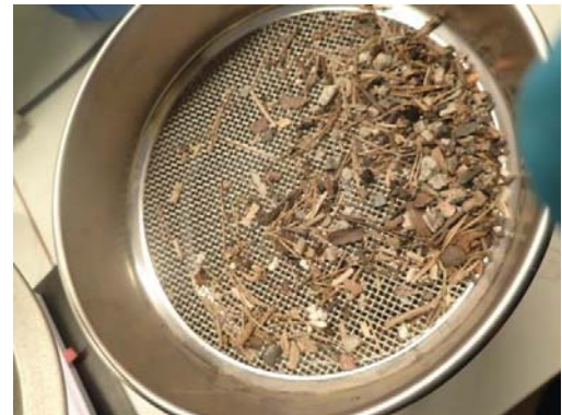
Figure 10: Sieving of samples through 8mm sieve and discarding debris
