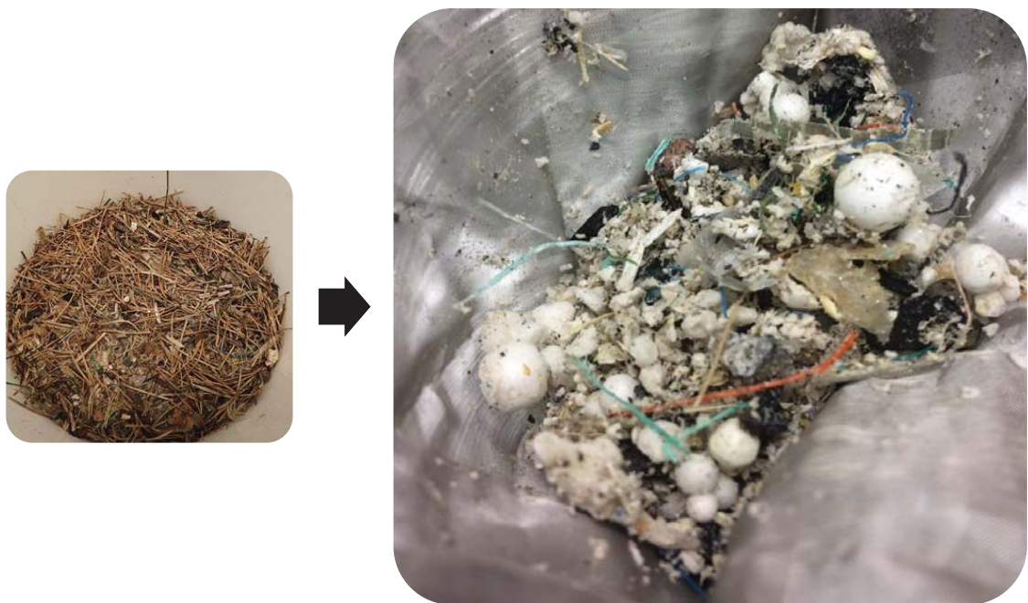
Figure 32: Microplastics and hard-to-digest debris material from Bygdøy sjøbad beach plastic debris samples after chemical digestion
