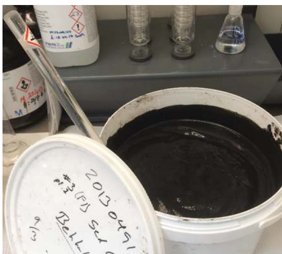
Figure 15: Homogenization of sediment sample (F1) from Bekkelaget WWTP. A long glass rod is used to mix the sediment well.
