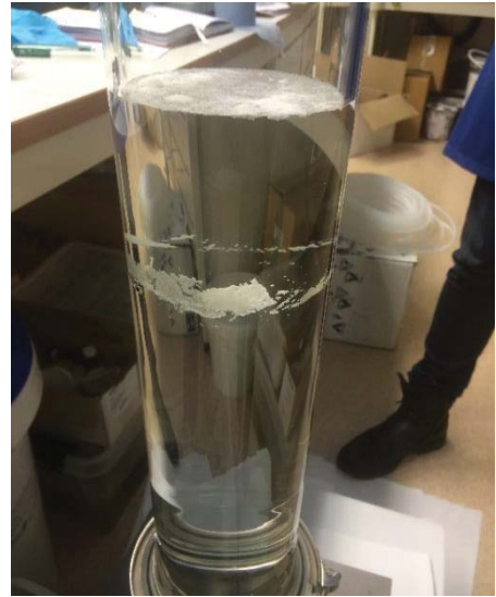
Figure 25: (Left) Introduction of PE powder in the separation chamber. \text{CaCl}_2 solution is filled from the bottom.
