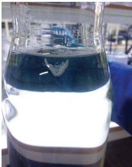
Figure 28: PET powder stuck to the constriction of the glass column when \text{CaCl}_2 was used as separation solution and sample was introduced from top.
