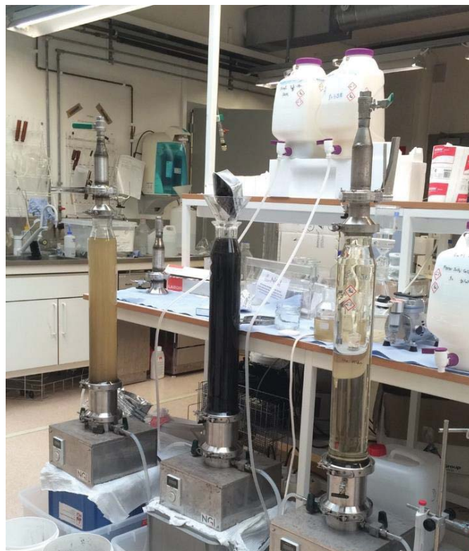
Figure 3: Three Bautas in running condition at NGI. The left-most Bauta (5:1) contains Bygdøy sjøbad beach samples; Bekkelaget sediment introduction is under process in the middle Bauta (50:1); the right Bauta (10:1) is being used for spiking of lab sand
