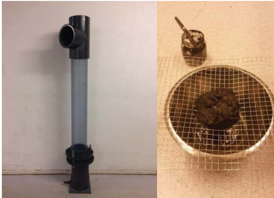
Figure 4a). The elutriation device used for extracting microplastics and b) a sediment sample container with a metal spatula and a 1 cm steel grate on top of a metal bowl. Photo a) personal; and photo b) by Thomas Botolfson.
