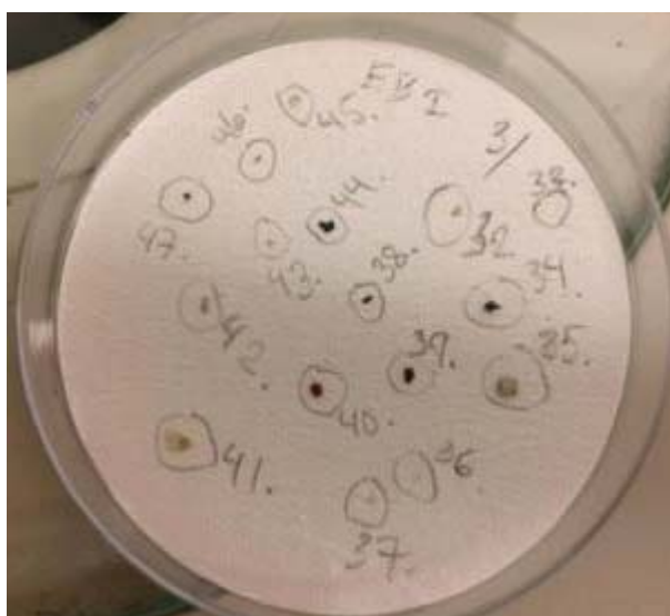
Figure 6. Petri dish containing a Whatman ® GF-F with particles suspected of being plastic polymers.
