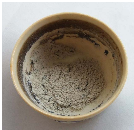
Figure 19 – The example of the struvite which was achieved under the different conditions, such as time (20, 40 and 60), pH (8.0; 8.3), ratio of Mg: N (1.2: 10; 1.5: 10)
