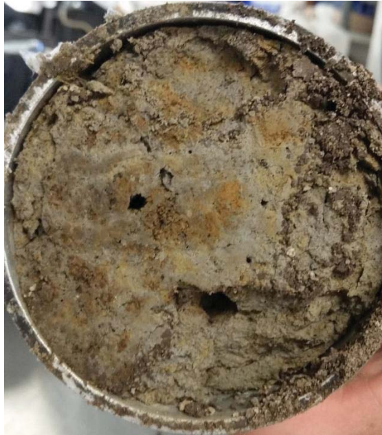
Fig. 7. Cross section of the bottom of a soil column from Kroer of the macroporous soil type Epistagnic Albeluvisol (siltic). Macropores, produced from biological processes are visible and connected to the open air at the bottom of the 20-cm column. Indication of rust stain colours the soil. Photo: Roger Holten
