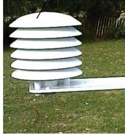
(b) A thermistor in a radiation shield.
