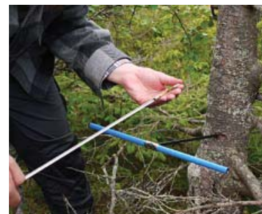
Figure 3 – Sample being taken with increment borer.
