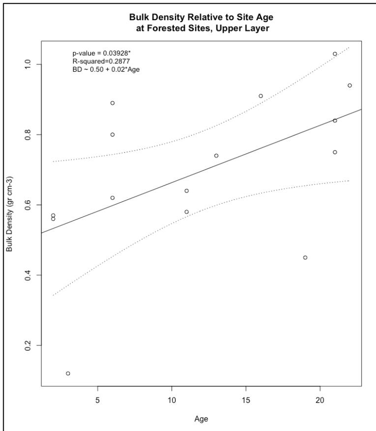
**Figure 14. Significant relationship between bulk density of upper layer soils relative to age at forested sites ( $p \leq 0.05$ ; CI = 95%, n = 15). Solid line = regression lines fitted to model with significant p-value; dotted lines = confidence interval.**
